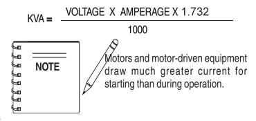
An inadequate size connecting cable which cannot carry the required load can cause a voltage drop which can burn out the appliance or tool and overheat the cable. See Table 5.
